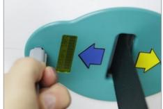
Perform a brief test to ensure proper connectivity. If the Hoist is OFF, turn it ON. Use the handset to RAISE and LOWER the carry bar. For powered traverse Hoists, also check the Hoist correctly moves FORWARD and BACK along the track using the handset. See section 'Hoist Operation' for details of how to perform these functions. If these operations all work as intended, then the handset is correctly connected to the Hoist.
