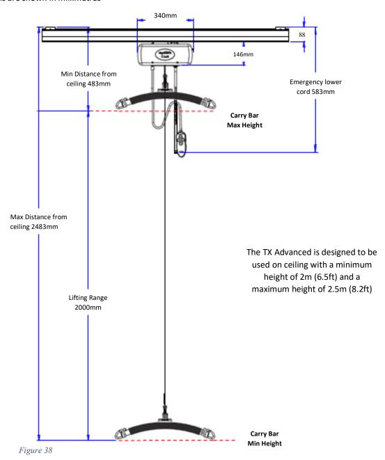
The diagram above (Figure 38) shows the relevant lifting ranges and dimensional sizes of the Hoist. The direction of travel can only be made within the boundaries of where the Hoist is in the track system.
