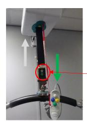
The Lift Tape includes arrows that corresponds with the colour scheme on the Handset to indicate the correct UP and DOWN button.
