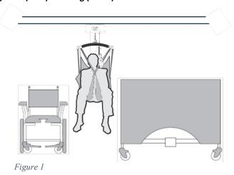
The TX Advanced Hoist is a Ceiling Track Hoist, and should only be used whilst on the Ceiling Track. It has the ability to raise up an individual from one location, such as a bed, move the individual along the track to another location and finally lower the individual, such as into a chair or a bath.
